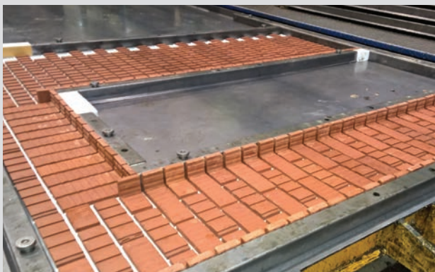
Complete Concrete Embedment Achieved with Dove-tail Key
