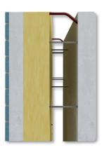
achieve the full monolithic construction of the reinforced concrete wall. The insulation will give a U value of min 0.25 W/m<sup>2</sup>C. Minimum wall thickness will be 300mm. Thicker walls can be accommodated and higher U Values on request.
