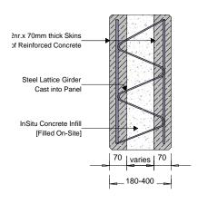
Single panel sizes will be up to a maximum height of 3.0m and length of 7.0m with larger panels being designed and manufactured on an individual basis. If the height has to be greater than 3.0m the panel can be turned through 90° and the length can then be used for the height required. This will result in more vertical joints being visible as the width cannot be more than 3.0m.
